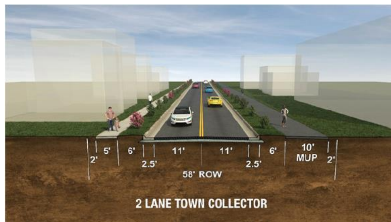
Cross Section 2- 2 Lane Town Collector Road
