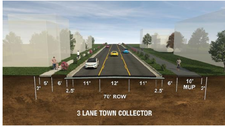
Cross Section 3- 3 Lane Town Collector Road
