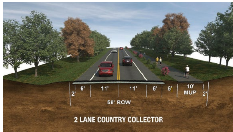
Cross Section 7- 2 Lane Country Collector Road
