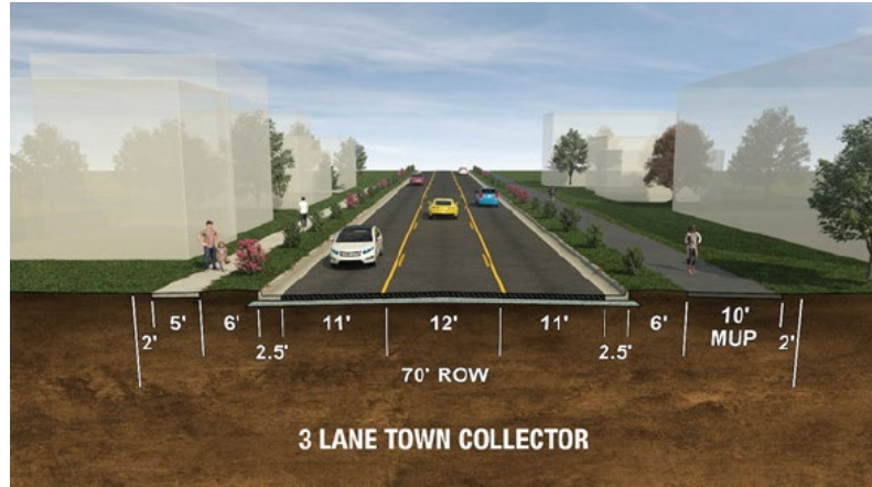
Cross Section 3- 3 Lane Town Collector Road
