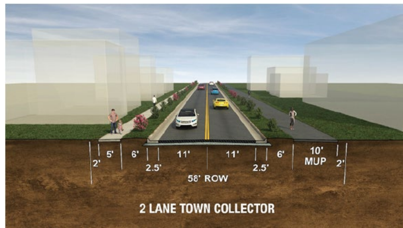
Cross Section 2- 2 Lane Town Collector Road
