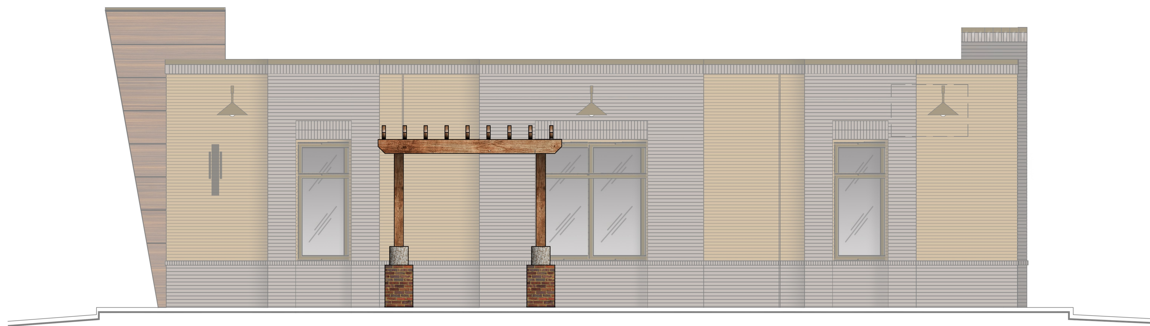
4 EAST ELEVATION WITH PERGOLA 1/2"=1'-0" 0 2 4 FEET
