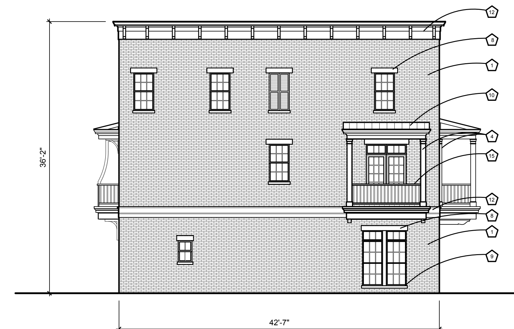
4 Live/ Work #1 Side Elevation 1/8" = 1'-0"
