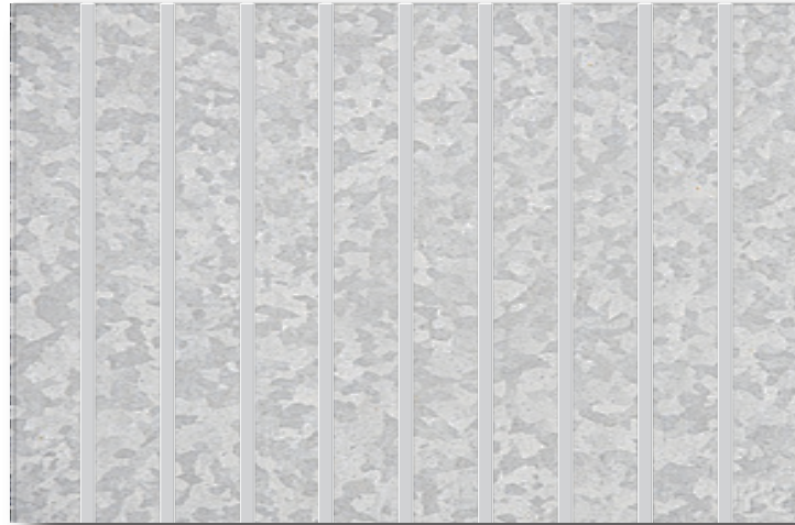
METAL ROOF: All Roof Structures, Trim & Downspouts to match Natural Galvalume Finish
